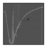
applied the brake pedal too long (part A), which resulted in wheel-blocking (point B).
